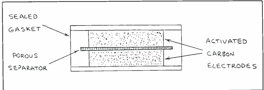
Fig. 1. Internal construction details of a super capacitor.
