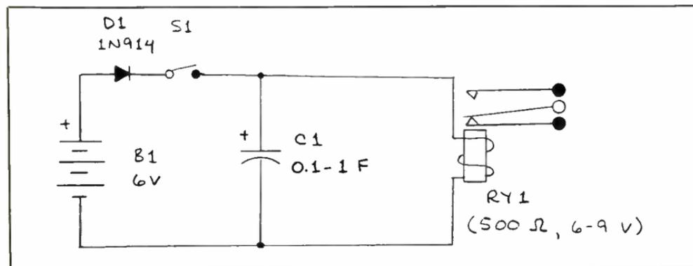
Fig. 8. An ultra-simple super-capacitor timer circuit.
