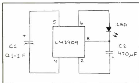
Fig. 6. Super-capacitor-powered LED flasher circuit.
