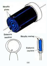
Tubular capacitors (A) are made by rolling strips of paper or plastic insulation sandwiched between strips of metal foil. Ceramic disc capacitors (B) are made by coating the faces of a ceramic wafer with a metallic film. than paper, plastic dielectric capacitors are smaller than paper units of the same ratings. But even the low-loss polystyrene capacitors aren't suitable for high frequency work because of selfinductance.
