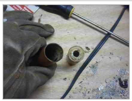
Now grab the core with a hooked dental pick, o-ring tool, or even a small bit of wire with a slight hook in it. Pull out your prize.
