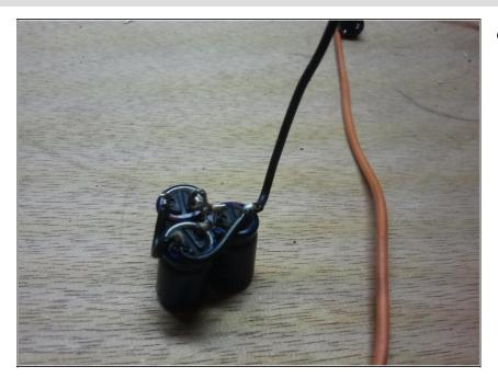
Cap bundle with the positives wired and the rest is now the pigtail for one of the positive leads.
