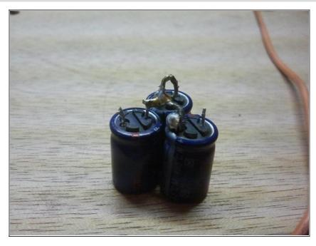
Now, here comes the fun part. Take the replacement value caps, for ME, alone, I used three 25uf@250v caps per side of the cap. Remember, CAPS IN PARALLEL ARE ADDITIVE, while keeping the working voltages the same. Yes, I purposely chose 3 caps because they will form a triangular pattern for better centering. I put a large loop on these negatives, since this will be the common point for the cap.
