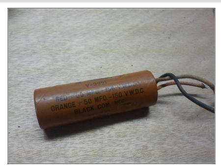
Let's start off with the offending part. A dual cap 50uf@150wvdc in a waxen pressed board container.
