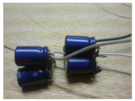
Take the negative lead from the second cap, and feed it through the center of the first cap, and cut it long enough to hook it to the first bundle's loop(remember that?)
