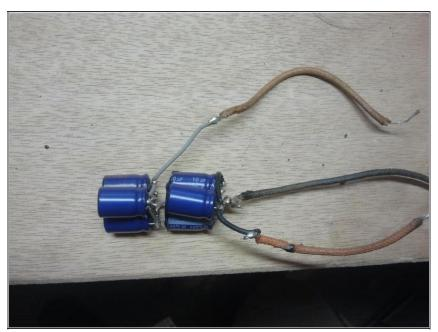
Reassemble the two cap bundles, soldering the negative lead from the second bundle, and the black(or whatever color it is) to the lug on the first bundle. Attach the remaining original wires to the positive leads.
