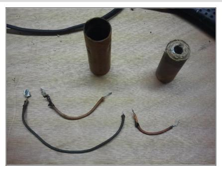
Here are your 5 constituent parts of the cap, less the plug material.
