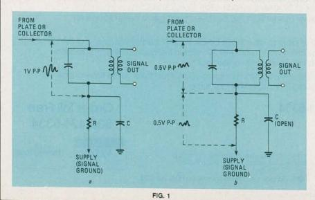
state sets, *don't!* Instead, turn the power off, tack in the substitute capacitor, and then turn the set back on. If the unwanted signal is gone and the symptom disappears, you've found the problem.
