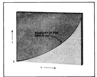
**2. Etched board.** Foil can have any pattern, to provide any increasing function of capacitance with overlap distance (x). For convenience in analysis, foil shown here covers area from y = 0 to y = y(x). Therefore overlap area is integral of y(x).
