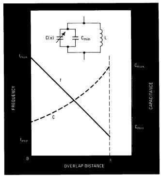
3. Linear tuning. To make resonant frequency of LC tank circuit change linearly with overlap, foil needs shape defined in text.
