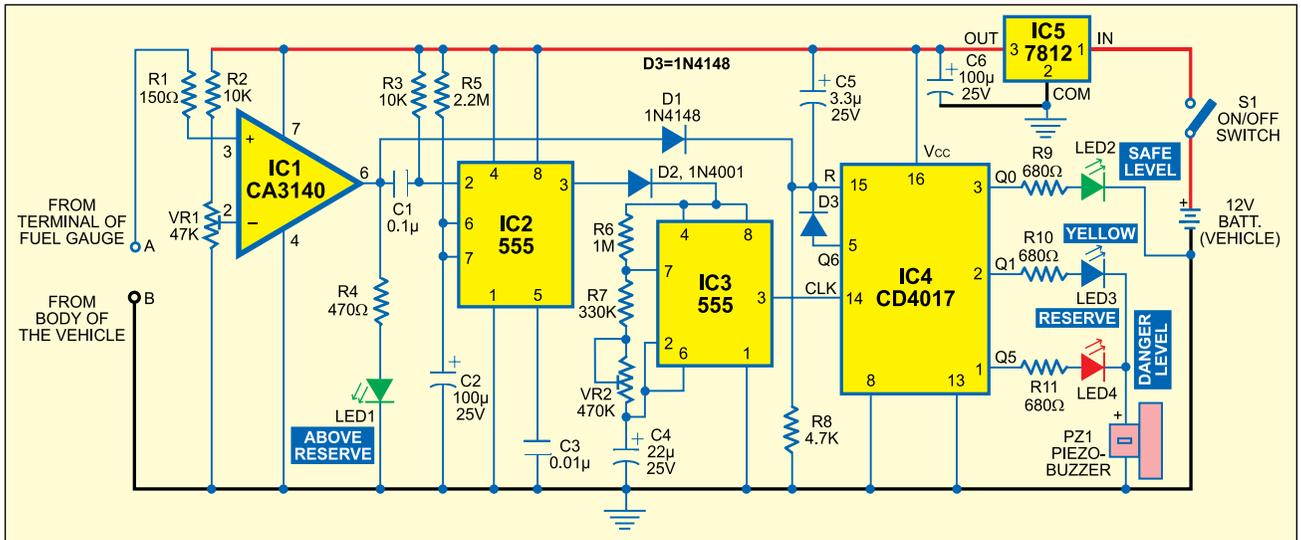
indication when the fuel level drops alarmingly below the reserve level, helping you to avoid running out of petrol on the way.
