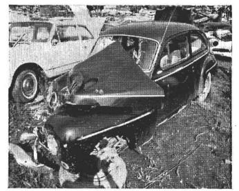
The driver of this European car survived a moderately severe frontal collision with the corner of a concrete wall, resulting in 24 in. of frontal deformation. The driver, age 23, 163 lbs., 5 ft. II in, male was wearing the three-point shoulder system tightly. His injuries consisted of a small laceration of the chin, a left clavicle bruise, left pneumothorax, abrasions on the right iliac crest, all probably related
