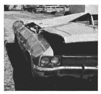
The untrained driver of this vehicle lost control of the car at 60 mph when she experienced a left rear tire blowout. The car left the roadway and rolled over two or three times. The roof deformation was 16 in, on the right side of the vehicle but all areas of the roof were deformed. The 29-year old, 123 lb. 5 ft. 7 in. female driver was using a lap and
