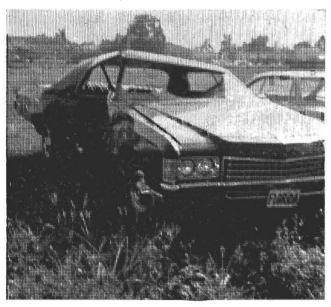
This 1971 Chevrolet four-door hardtop proceeded to cross an intersection after stopping at a stop sign and was struck in the right side by another passenger car traveling 60 mph. Exterior deformation was about 25 in. The driver was the only occupant in
