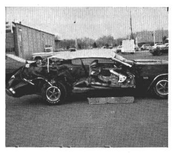
The vehicle in this case was attempting to pass a car traveling 50 mph, pulling a four-wheel farm trailer loaded with corn. The trailer began to whip and "fishtail" and was struck by the overtaking car causing 13 in. of deformation into the right side and the tearing away of some of the side structure. Only the two rear seat occupants, of the four occupants in the car, were injured. The driver, a person of small stature, was unrestrained
