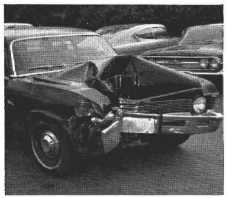
The driver of this vehicle fell asleep as his vehicle was entering a curve. The 1969 Chevy II struck a concrete bridge abutment at an estimate speed of 35 mph resulting in a frontal crush of 20 in. The lone occupant, who was a 23-year old, 6 ft. in., 210lb male, wearing a lap-shoulder belt, had bruises on both knees,
