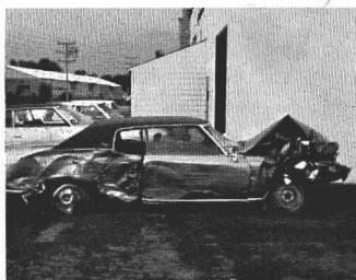
This 1971 Chevrolet left the road on a curve, struck a large mail box, struck a 20-in. dia. tree with the right front corner of the vehicle, continued on side-swiping three more 20-in. dia. trees with the right side of the vehicle before eventually coming to rest. Multiple impact collisions such as this accident can force an unrestrained occupant from the area where he has the
