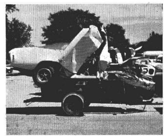
The next case is an unusually severe, single-car collision, headon with a concrete bridge. Vehicle deformation was 95 in. Note that the right front wheel has been forced back into the rear seat area. The driver of the vehicle alleges that he was dodging an oncoming truck that was passing another truck. The driv-
