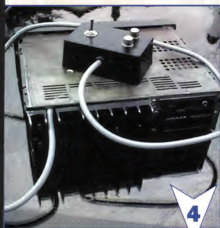
Rear view of the modified Kenwood head unit. The unusual cable exit point on the back of the device is deliberate - this unit is 'removable'. This is one of the reasons for specifying the in-line DIN connections that can be seen to the left of the picture.
