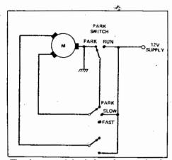
The wiper control circuit shown is conventional on most makes. The Delay unit is installed in the 'slow speed' circuit, but slow wipe is still possible by turning the delay to zero.
