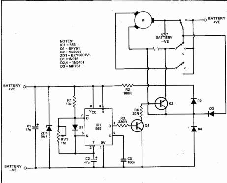
The circuit uses a 555 timer in the astable mode to provide the delay function. The unit is connected into the slow speed wiper circuit at the points indicated by the breaks.
