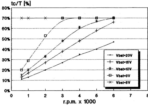
Fig. 9 - Conduction angle versus r.p.m.
