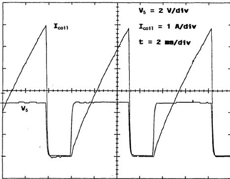
Fig. 6 - Duty-cycle = 70%; frequency = 140 Hz.
