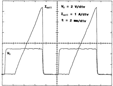
Fig. 5 - Duty-cycle = 70%; frequency = 100 Hz.
