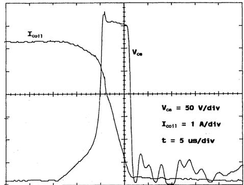
Fig. 7 - Turn-off in normal operating mode.
