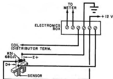
Fig. 5. External connections to the ignition monitor.
