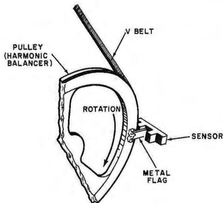
Fig. 3. Metal flag,  $\frac{5}{8}$  in. by  $\frac{1}{4}$  in. is attached to rim of harmonic balancer pulley to pass through slot in sensor interrupting light beam.
