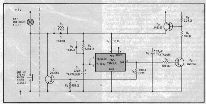
Holds the light. When car door closes, output current pulse from 555 timer turns on transistor Q<sub>1</sub> to keep interior light on for about 10 seconds. This type of one-shot arrangement, driving the line that is sensed, can be added at any point in the circuit. It is useful in alarm systems, process controls, automatic machinery, safety circuits, and convenience circuits such as this one.
