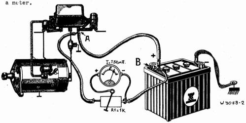
The meter should have a sensitivity of, say,  $50\mu A$ . Less sensitive meters can also be tried, but how well they work will depend on the voltage drop across the battery cable. A good type of meter to use is one with a centre zero, so that the pointer can deflect in different directions for discharge and charge conditions.
