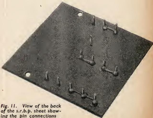
Fig. 11. View of the back of the s.r.b.p. sheet showing the pin connections
