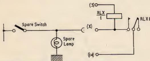
Fig. 5b. Basic circuit of an "add-on" system
