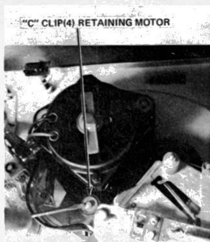
FIG. 6—C CLIPS hold the motor in place. Remove them, then the motor, to get at the upper motor bearings.
