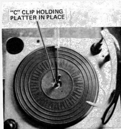
FIG. 1—TYPICAL RECORD CHANGER. Note that there is usually only a single C-clip holding the platter in place.
