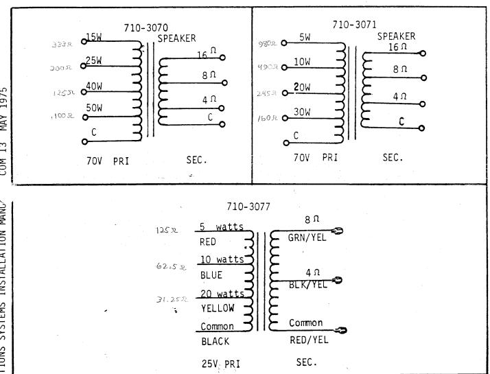
NOTE - The above values are based on a rated secondary load. With a sixteenohm load connected to the eight-ohm winding, primary impedance values are doubled. Power ratings are then divided by "2".
