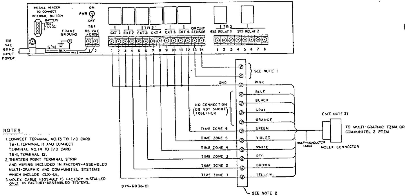
Control Circuit Wiring Diagram for Six-Circuit Time Signalling
