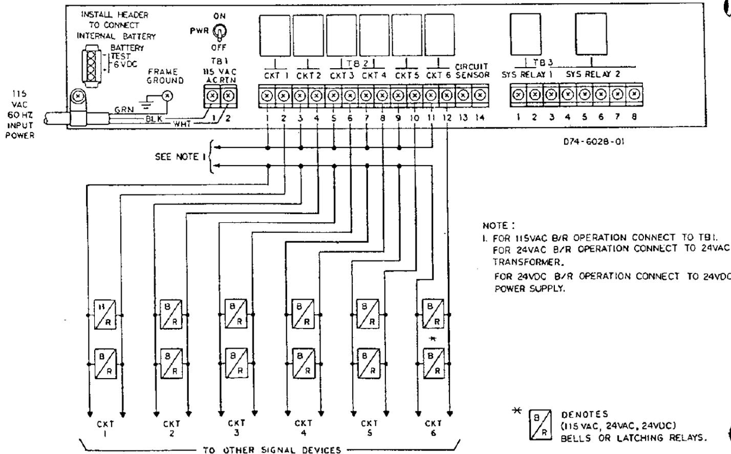
Control Circuit Wiring Diagram for Ancillary Signalling and/or
