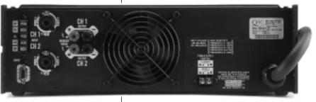
The amplifier shall employ forced-air cooling with a variable speed fan for minimum acoustic noise. Air flow shall be from rear to front to avoid temperature rise inside the rack. Rack mounting shall be possible without clearance between amplifiers for ventilation. The amplifier shall be capable of continuous operation at 1/3 power, into four-ohm loads, for ambient temperatures up to 104° F (40° C).
