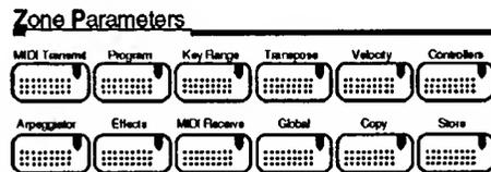
The **Global** button is especially important to servicers. Entering the **Global** menu will allow you to save the customer's setups, reset the PC88 and enter MIDIScope. It will also allow you to check the available memory and "All Notes Off" command, etc.
