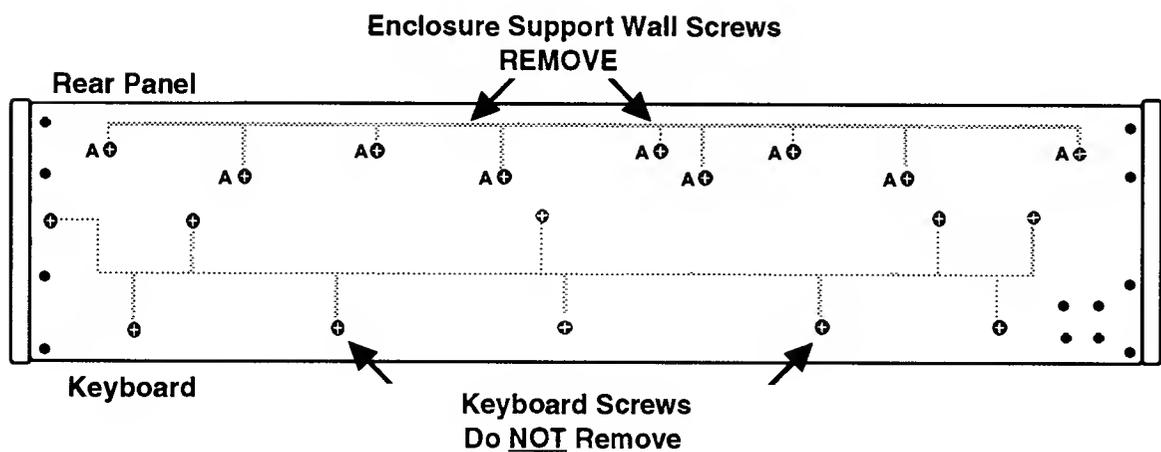
Remove the 9 screws labelled A. Turn the unit over into playing position.
