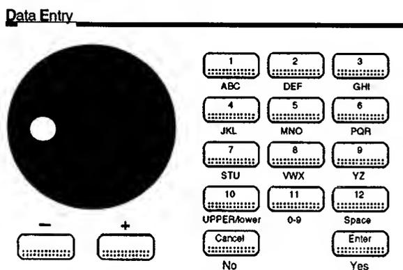
The Alpha Wheel is used to quickly move through voices and setups. In the Parameter mode, you can quickly move through parameters.
