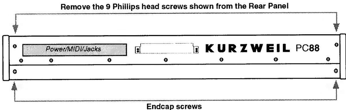
*Enclosure Support Wall**Removing the Top Cover Assembly*
