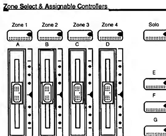
Each button has a three color LED. A green LED is lit when the zone is on or active, an orange LED when it is muted and a red LED when it is being soloed.
