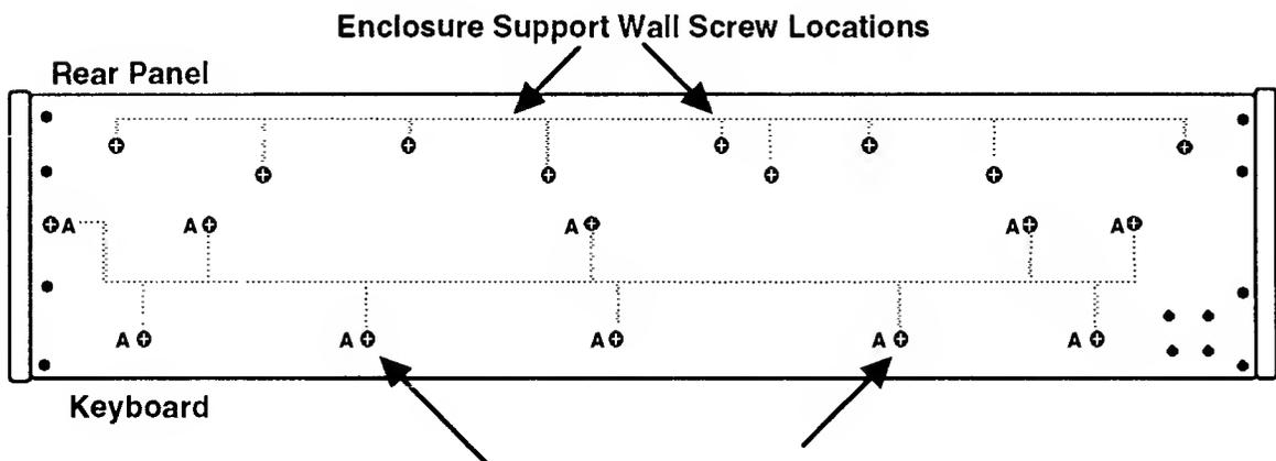
Tilt the bottom chassis up and remove the Phillips head screws located closest to the rear panel.
