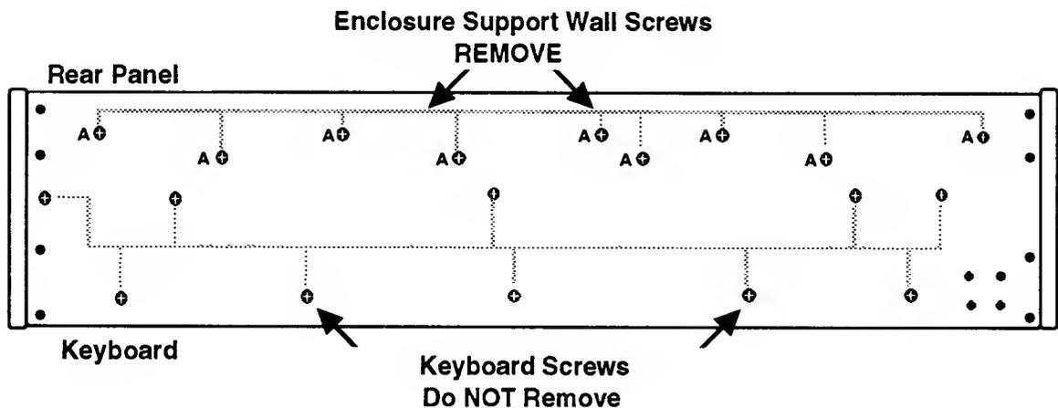
If the unit does not have screws in these locations, the unit contains EMI Shields. Please follow the Disassembly/Assembly Procedures for units containing EMI Shields. These instructions begin on page 3-4.
