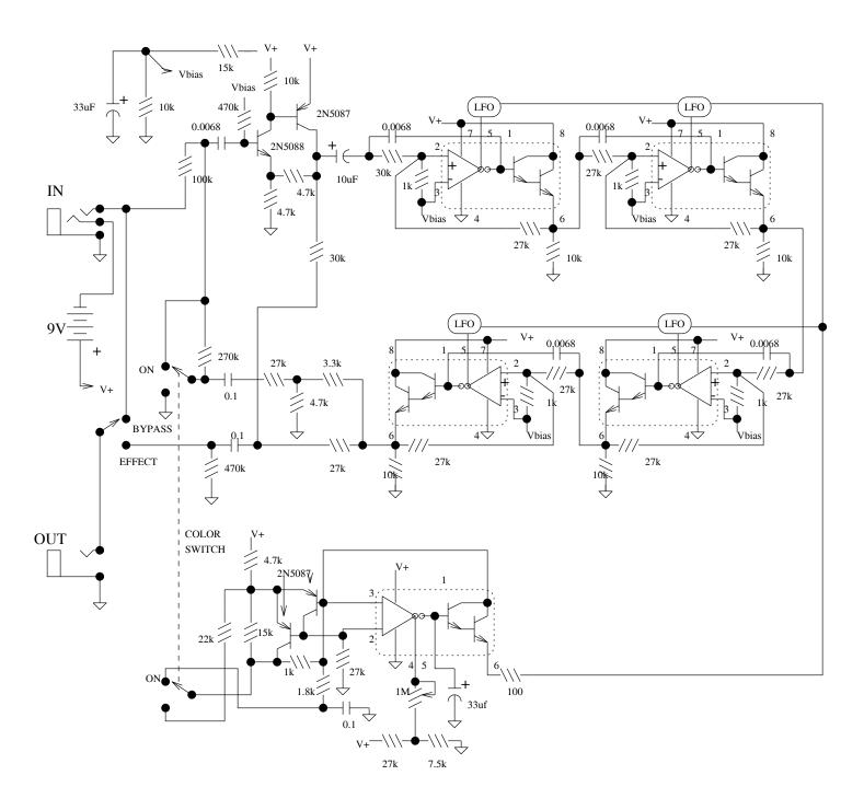
The Small Stone is somewhat unique in using Operational Transconductance Amplifiers (OTA's) for phase shift stages instead of opamps with variable resistors. All of the IC's are house marked EH1048, but can be replaced with CA3094 which is a combination of an OTA equal to the CA3080 and a darlington emitter follower. Later Small Stones used slightly different circuits, but all used the OTA.
