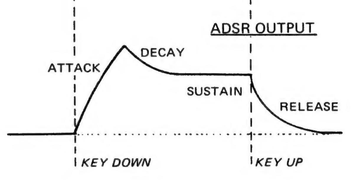
NOTE: The ADSR is initiated with a gate and trigger voltage, and the AR envelope requires only the gate.
