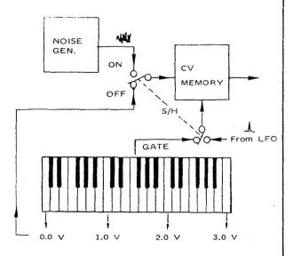
The voltage on S1A pin 2 charges up the memory capacitor (C13) through Q5. Q5 is turned on by the Gate generator or the LFO trigger pulse through CR4. Q6 and Z1A are an FET op amp follower with high input impedance to buffer the voltage on C13. The output of the Keyboard Control Voltage Memory circuit is supplied to the control inputs of the VCO and the VCF via J4-1 and J4-3.
