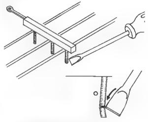
CAUTION: IMPROPER ADJUSTMENT WILL CAUSE SPRING BREAKAGE.
