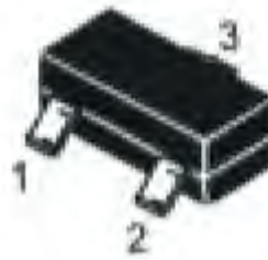
2N3904; NPN Transistor (SOT23)
