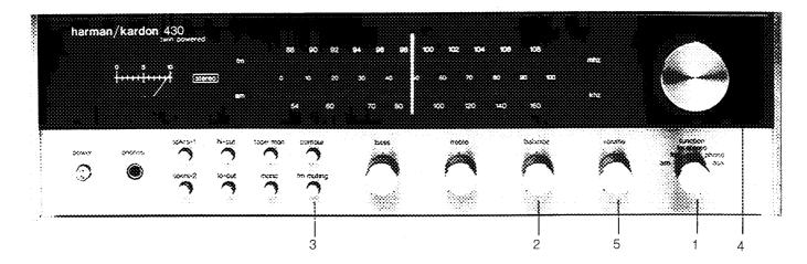
Five basic controls are used to receive FM broadcasts through the 430: FUNCTION, VOLUME, BALANCE, TUNING, and FM MUTING. Make the following adjustments to these controls after activating the SPEAKERS 1 switch:
