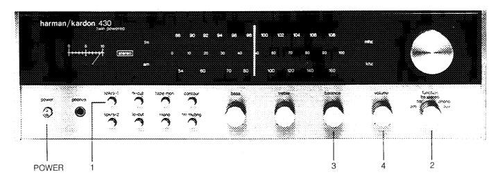
Familiarize yourself with the front panel controls. There are six knobs and nine pushbuttons controlling all the features of the receiver. Each of the controls performs a different function, but instead of discussing each control separately, we will illustrate how they work together to control the reproduction of sound through the 430. Find the VOLUME control and turn it down (counterclockwise). Push the POWER switch to turn the 430 on.
