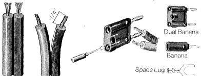
For your convenience, the output terminals of the Citation 16 accept spade lugs, banana plugs and dual banana plugs in addition to bare wire. Enclosed with your unit are two dual banana plugs — one for each channel.
