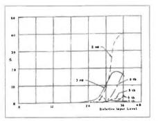
Figure 1. Distortion components for two-stage triode amplifier.
