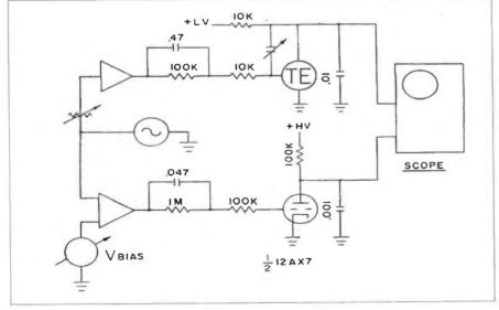
Figure 10. Comparison Tester for 12AX7 verses a Tube Emulator
