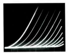
Figure 9. Output (plate) characteristics of a 12AX7 triode tube emulator: Horz: 5 volts / div, Vert: 0.5 milliamps / div, Step: .05 volts
