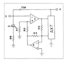
Figure 7. Low- noise Tube Emulator for a 12AX7
