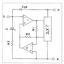
Figure 6. Complete Tube Emulator for a 12AX7
