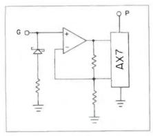
Figure 8. Non-Inverting Tube Emulator
