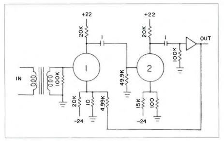
Figure 21. A microphone preamplifier using triode tube emulators.
