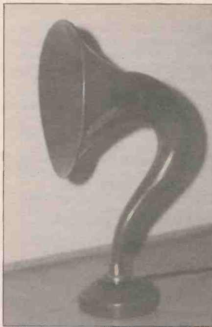
Photo 1a. Sterling 'Baby' horn with diaphragm transducer. About 1924.
