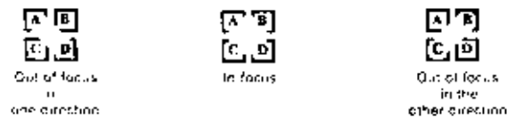
Figure 5.29 A method of developing the focus error signal.
