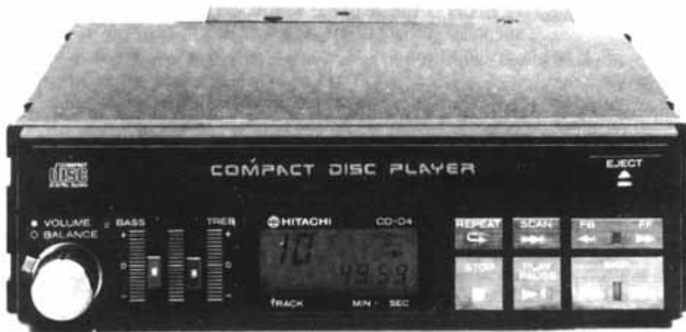
Figure 19.9 Hitachi's CD-D4 compact disc player uses anti-vibration techniques for improved sound quality.
