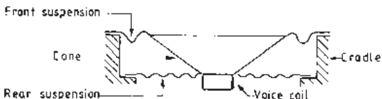
Figure 15.13 Moving coil loudspeaker cone, suspensions, voice coil assembly.
