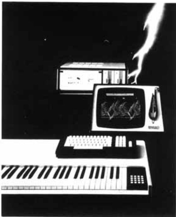
Figure 20.16 The Fairlight Computer Musical Instrument – the original studio sampling keyboard.
