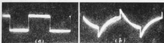
Fig. 5. Effect of phase distortion on a square-wave signal after passing through a reactive network in which there is no variation of attenuation with frequency. Repetition rate, 300 per sec.
