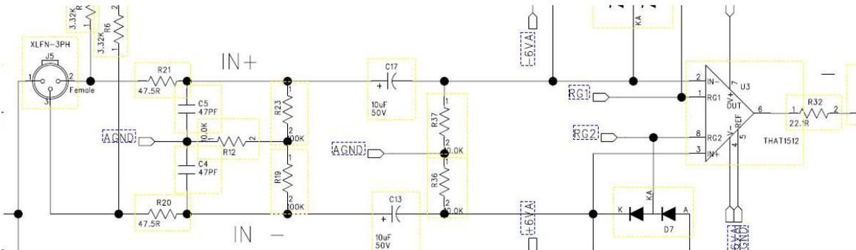
It can be seen the Pin 2 input is feeding the IN- pin on U3 which results in inverted phase on the output indicated by - sign. The reason for this inversion was that it was found that when the entire product was designed with the + in feeding IN+ the loop send was out of phase. Swapping the inputs of U3 was the easiest thing to do to bring the loop send int phase. It must be noted that U3 is a
