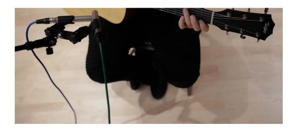
Most often, two mics will be set up, with one pointed toward the sound hole to pick up the lower frequencies, and the second mic pointed toward the neck and fingerboard to pick up the attack. Of course, the guitar's frequency range covers several octaves, which means a wide range of different audio wavelengths. Since the mics are a fixed distance from the source, those different waves will arrive at the mics at different points.
