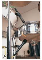
When miking a snare from above and below, the two signals will be out of phase, so use the polarityinvert switch on your desk (or in your DAW) on one of them.
