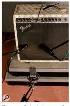
Phase cancellation isn't necessarily a bad thing. The 'phase EQ' technique uses three mics positioned to form a triangle. The faders on the desk (or in the DAW) can then be raised or lowered for each signal, altering the phase relationship between the signals — and this can be a less intrusive alternative to conventional EQ.
