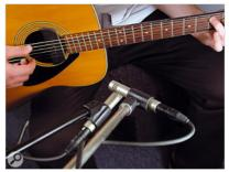
Phase can be a problem with stereo miking of sources that aren't stationary. An acoustic guitar player, for example, will usually move the guitar at least a little during performance — which is why closely placed coincident pairs tend to be preferred over spaced stereo techniques.
