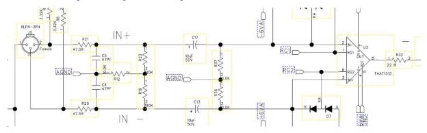
It can be seen the Pin 2 input is feeding the IN- pin on U3 which results in inverted phase on the output indicated by - sign. The reason for this inversion was that it was found that when the entire product was designed with the + in feeding IN+ the loop send was out of phase. Swapping the inputs of U3 was the easiest thing to do to bring the loop send int phase. It must be noted that U3 is a
