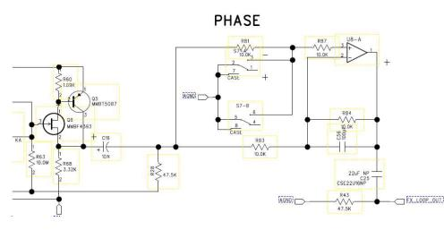
Normally 2 op amps are used to have an in phase and out of phase signal to chose from in making a phase inversion switch. In this circuit when the phase switch is in the rest position, open the when phase of the output is in phase with the input. This is
