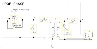
Here in the effects send circuit we always show the switches in the OUT position. In this case for a phase switch it is the position where the signal stays in phase Thus there are + signs on both sides.
