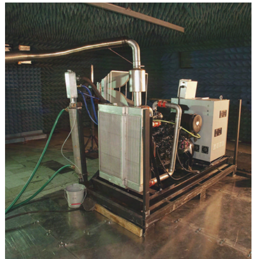
Figure 6 Chambers for MIL-STD 461-compliance tests don't need turntables; cables for these tests can run on the chamber floor (courtesy Dayton T Brown).
