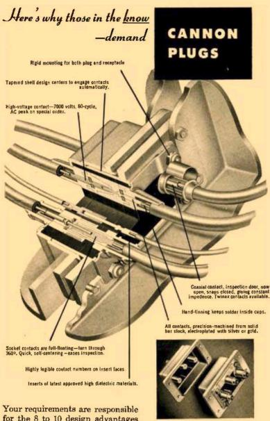
Your requirements are responsible for the 8 to 10 design advantages found in each type of Cannon Plug. That's why engineers know the specification is right when it calls for CANNON. The DP Connector Series is just one of many Cannon types — world's most complete line. Request bulletins by required type or describe connector service you need.
