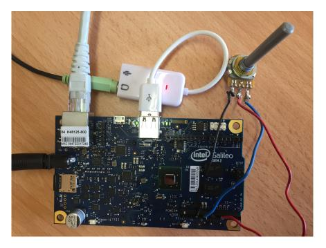
Figure 2: The Intel Galileo (GEN2) with ethernet, USB audio and a potentiometer connected to analog input 1 (pin A1)
