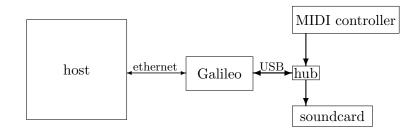
Figure 3: The Galileo Synthesizer layout
