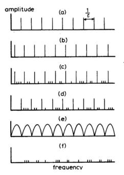
the single comb-filter distortion measurement method: (a) spectrum of pseudo-random binary sequence; (b) the same p.r.b.s. frequency shifted; (c) signal from system under test, showing distortion products in gaps; (d) signal re-shifted; (e) response of comb-filter for removing comb spectrum of p.r.b.s. test signal; and (f) comb-filter output. is repetition period of p.r.b.s.)
