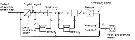
Fig. 5 (above). Analyser for output signal from system under test in double comb-filter method. Levels of test signal and distortion producta are measured on a p.p.m.
