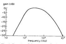
Fig. 4. Test signal frequency shaping characteristic.
