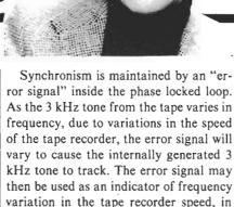
The phase locked loop is largely immune to variations in the amplitude of the tone from the tape, and it's capable of acquiring lock even when the incoming tone and the internal VCO are quite different in frequency.
