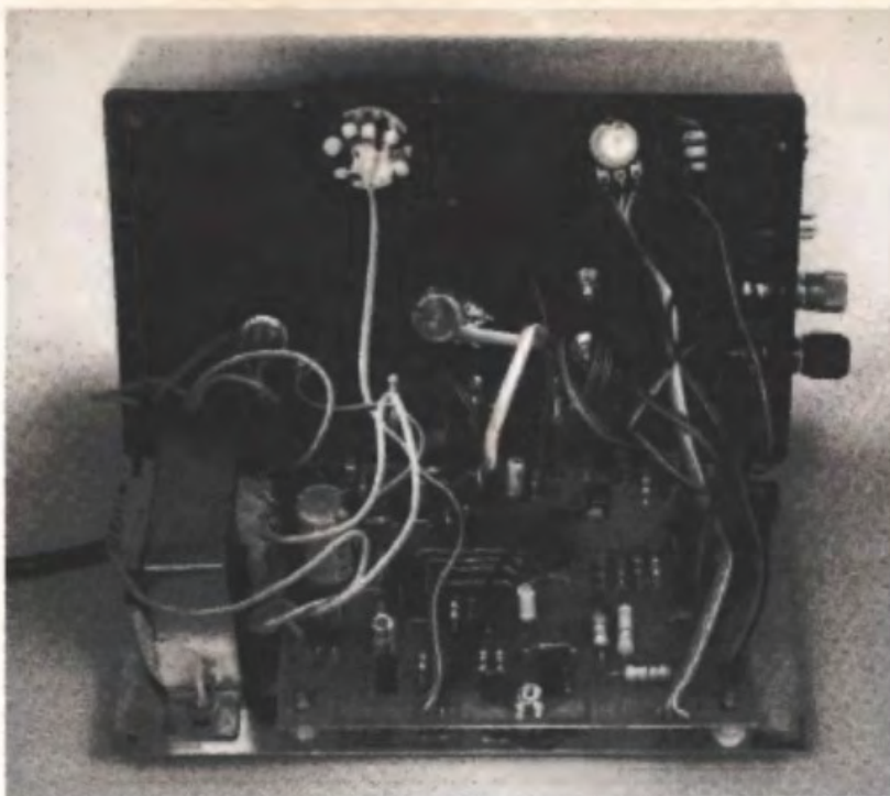
The wiring inside the Tone Burst Source is a bit of a bird's nest but is fairly straightforward if rainbow cable is used. Don't bind the wires together as this could create crosstalk problems.
