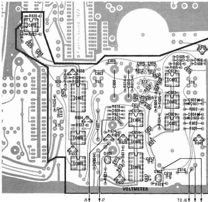
FIG. 12—COMPONENT LAYOUT diagram for the voltmeter. Parts used in this section are coded with numbers in the 600 series. See Fig. 10 for the schematic diagram.
