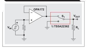
The switch on-resistance forms a voltage divider with the load resistance  $R_L$  and the output voltage is:
