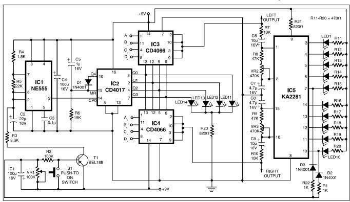
ing through the channels continues until it receives an audio signal exceeding the preset threshold value. The skip switch S1 is used to skip a channel even if audio is present in the selected channel. The number of channels can be easily extended up to ten, by using additional  $4066\ \mathrm{ICs.}$
