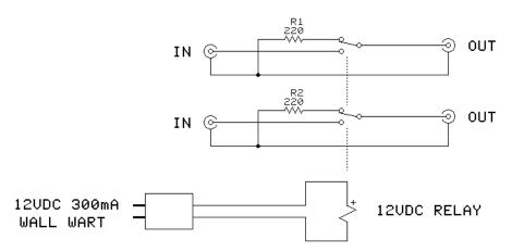
THIS CIRCUIT WILL DISCONNECT THE INPUTS OF A POWER AMPLIFIER FROM A PREAMP OUTPUT TO PREVENT HUM AND BUZZ IF THE AMPLIFIER IS ALWAYS LEFT ON, OR IS ONE OF THE SIGNAL SENSING "AUTO-ON" TYPES. ALWAYS ON TYPE POWER AMPS OR SUBWOOFERS CAN HUM IF THE DRIVING UNIT IS POWERED OFF, AND THE OUTPUT CIRCUITS ARE HIGH IMPEDANCE. SIMPLY PLUG THE 12VDC WALL WART INTO THE SWITCHED AC POWER OUTLET ON THE PREAMP OR RECEIVER.
