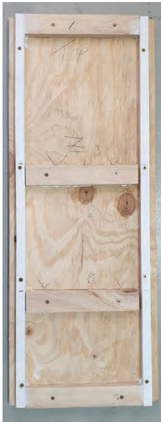
Fig.17: the subwoofer panels are cut from three 600 x 1200mm sheets. As with the monitor speakers, you can cut two of the sheets down the middle. So you don't need to purchase a fourth sheet for just one panel, the last piece is made from one of the bookshelf speaker off-cuts (see Fig.13, last month).
