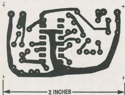
Fig. 3. The transmitter's printed-circuit layout is shown here at full size.
