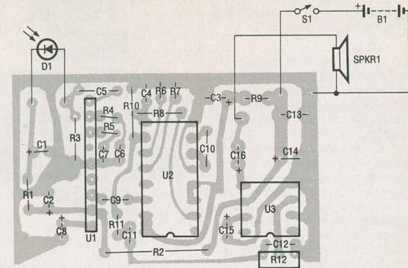
Fig. 6. The receiver's printed-circuit board should be assembled using  $\frac{1}{8}$ -watt or smaller resistors and miniature (radial lead electrolytic and ceramic-disc) capacitors. The volume control (R12) can be a miniature PC-mounted potentiometer or conventional unit, which would have to be mounted off-board.
