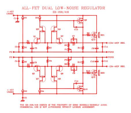
Fig. 2. The EB-208/418 ALL-FET Wide-band, Low-noise regulator.
