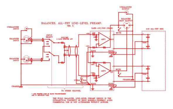
Fig. 4. Two EB-107/309 amps wired for balanced operation, using 4-gang stepped attenuator
