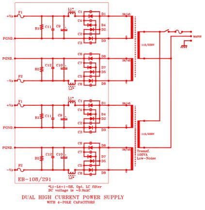
Fig. 3. The EB-108/291 High Current Power Supply.
