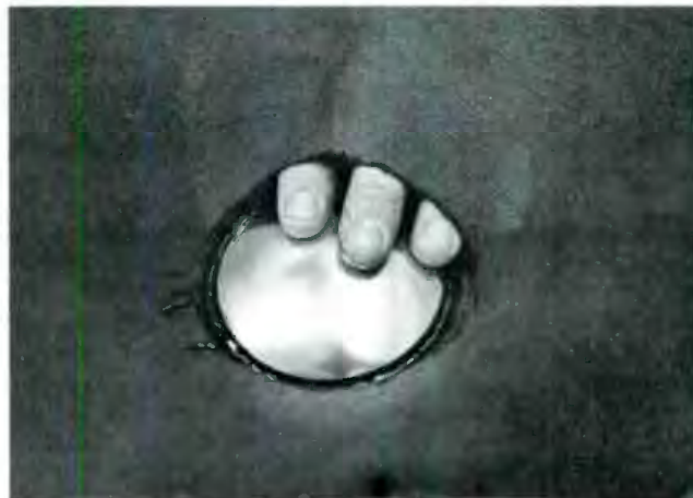
This one definitely needs a re-coning job. Just another example of what can happen when the SPL goes up.
