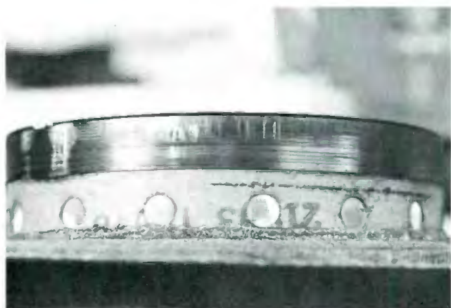
A new voice coil on its bobbin, partially coated with ferrofluid.
