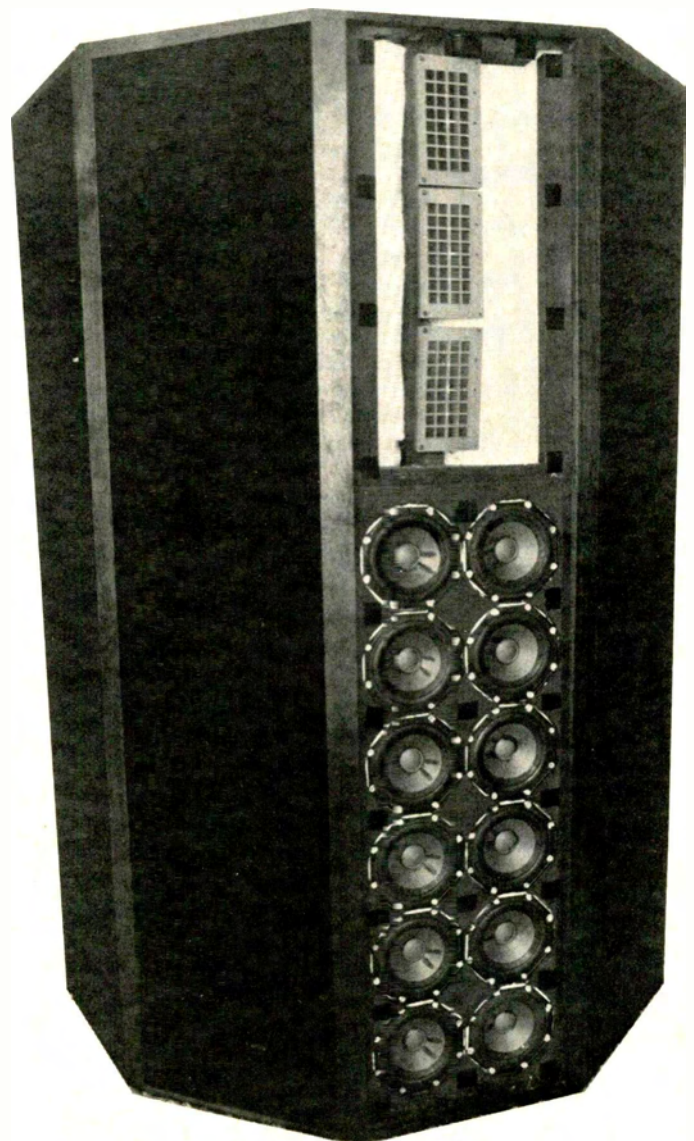
Fig. 2—Photograph of one loudspeaker of an experimental stereo pair designed for inaudible modulation distortion. The enclosure is in the shape of a regular, right, decagonal cylinder. The foam grill has been removed from one of the five identical radiating surfaces to show the three electrostatic elements and twelve dynamic drivers located on each of these surfaces.
