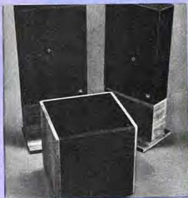
JBL L212 has mid/high-frequency "satellites" and common bass module.
